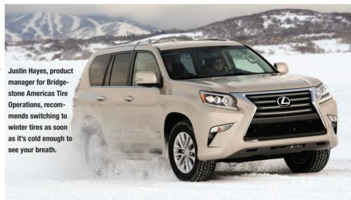
or snowball—you want your winter tire to store some snow in those slots and sipes to maximize your tire's grip in snow," adds Hayes. "On ice, which is slippery due to the incredibly thin layer of water on top of it, a tire engineered with Mutli-Cell compound soaks that water up like a sponge so the tire makes contact with the ice."
